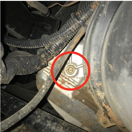
11. Find and remove drain plug on the drivers side in front of clutches.
