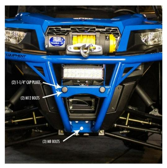
3. Install 1-1/4" Cap Plugs into the tubes located at the middle bracket.
