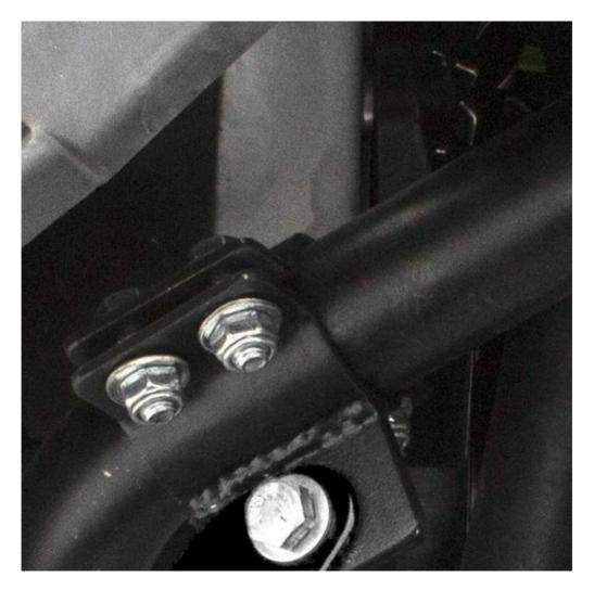
6. Using the supplied hardware, attach the Mounting Arms to the Clamps, then to the Front Bumper Tabs.
