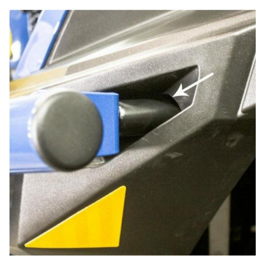
5. Install the supplied (2) 1-½" bar clamps using the supplied (8) M8x25 Hex (16) ¼" washers (8) M8 Nylocks
