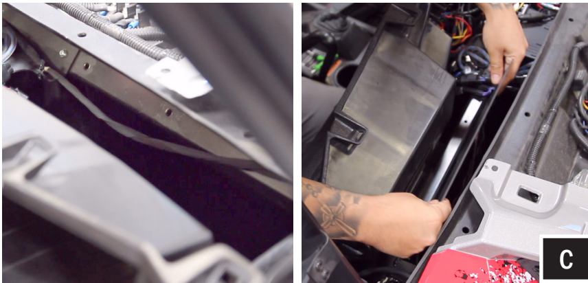
C. For this step you will need the sub enclosure mounting plate as well as two (2) M5 screws, two (2) 8mm nuts and four (4) M5 washers. Place the mounting plate on the factory dash cross member bar behind the glovebox. Match up the holes from the plate and the bar to insert the M5 screws and washers from top. Use the 8mm nuts and washers to fasten from underneath.
