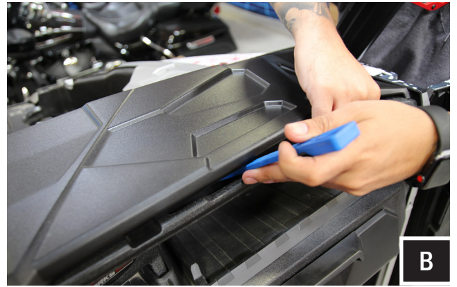
B. Using a panel removal tool, pry top of dash panel to unclip and remove.
