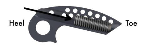
For Elevation above 5,000 feet use one size smaller set screw. If it calls for long screw, use medium If using 32 inch or larger tires use the GOLD BIG TIRE secondary spring for stock or tuned machine
