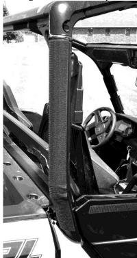
7. Now move to the top of the door. Starting at the front place the 12" along the top of the door on the outside. Then follow the different angles of the door and place two 10" strips then a 12" strip. As shown on the next page.
