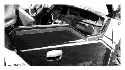
8. After all the Velcro is in place take the door and place it on the vehicle. The following series of photos show how it should look after being installed.
